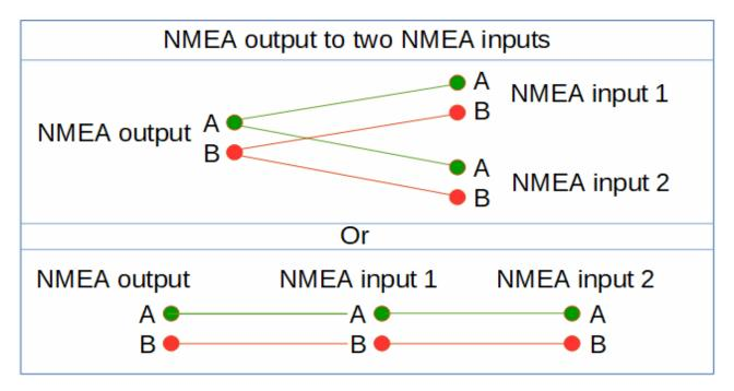
Please note that not all NMEA0183 devices follow the standard! Some devices have a single-wire talker, or a single-wire listener instead of the two-wire differential signals of the standard. These
